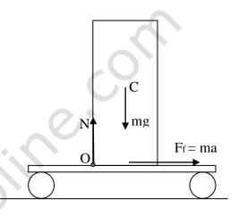
If the acceleration a of the cart is such that the compressor is just not tipping i.e. at the verge of tipping the torques due to the normal reaction and due to friction about the center of mass of the compressor are just balancing. Gives us
